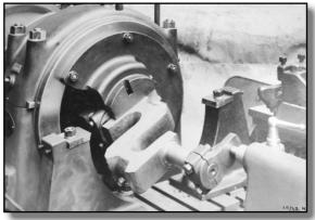
A crankshaft ready for machining in one of Gardner's own crankshaft turning machines.
